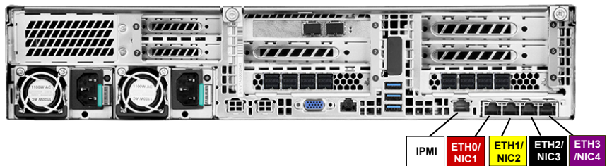
Figure 1-8 3340 Appliance rear port color codes
