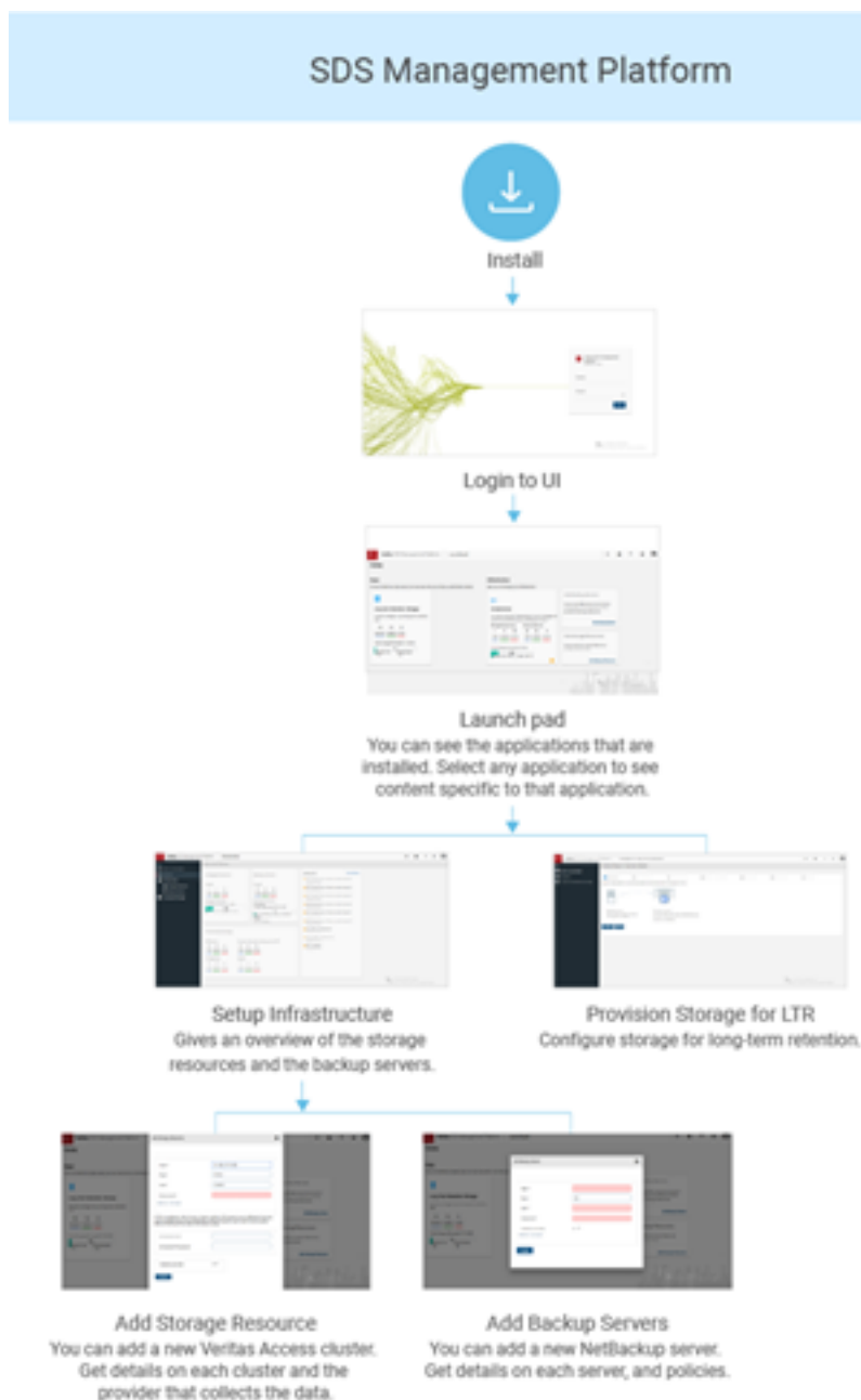
Figure 3-1 SDS Management Platform workflow
