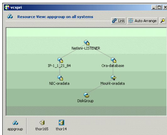
Figure 13-4 Example: A single-instance Oracle database is configured as a VCS service group (appgroup) on a two-node cluster
