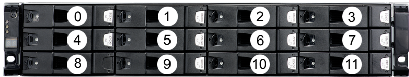
Figure A-1 Veritas 2U12 49TB Storage Shelf disk drive slot layout
