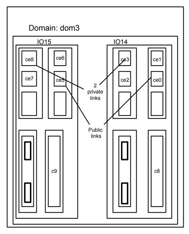
For e12K/15K/25K: In the following scenario, a cluster consists of the dom3 and the S6800f0 domains. The cluster is running service groups on the dom3 domain, which includes I/O boards IO14 and IO15. IO15 requires dynamic reconfiguration because of a malfunctioning component. The domain S6800f0 includes I/O boards IB8 and IB6. The disk controllers and NICs are labeled in the following diagrams.
