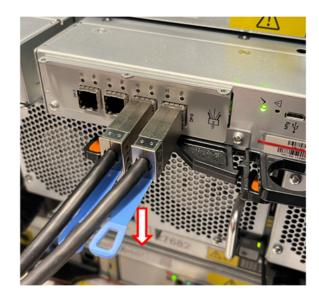
4 After labeling each cable, disconnect the SAS3 cables from the faulty SAS3 RAID controller.
