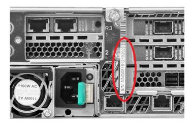
• For the 3360/5360/5362 Appliance, the serial number is located on the rear panel of the appliance above PSU 1 and begins with letters VTAS.
