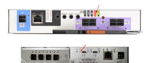
**Note:** A SAS3 RAID controller uses SAS3 cables. It may also have a SAS3 cable attached to it if there is a 5U84 Expansion Storage Shelf as part of the Appliance system.
