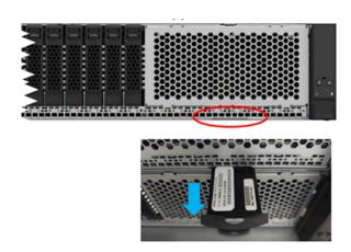
If the work order provides the 5U84 Storage Shelf serial number, verify that the serial number on the work order matches the serial number on the storage shelf. The Veritas Serial Number label is located in the lower right-hand corner of the shelf's rear panel under the power supply. Do not use the label in the upper left-hand corner for the Veritas Serial Number.
