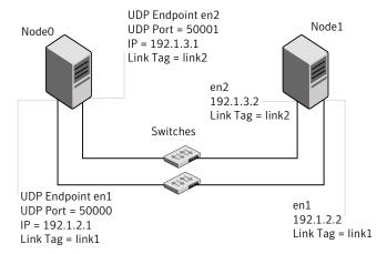
The configuration that the /etc/llttab file for Node 0 represents has directly attached crossover links. It might also have the links that are connected through a hub or switch. These links do not cross routers.
