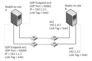
The configuration that the following /etc/llttab file represents for Node 1 has links crossing IP routers. Notice that IP addresses are shown for each link on each peer node. In this configuration broadcasts are disabled. Hence, the broadcast address does not need to be set in the link command of the /etc/llttab file.
