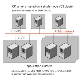
Figure 8-5 displays a configuration using a single CP server that is connected to multiple application clusters with each application cluster also using two coordinator disks.
