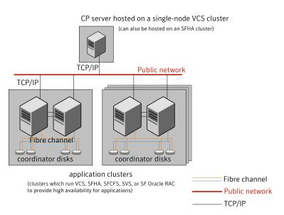
Figure 8-6 displays a configuration using a single CP server that is connected to multiple application clusters.
