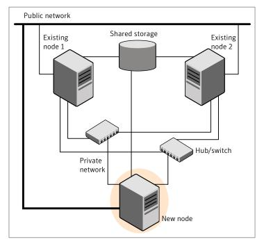
Figure 30-1Adding a node to a two-node cluster using two switches
