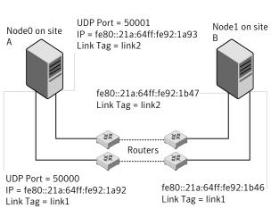
Figure J-4A typical configuration of links crossing an IP router
