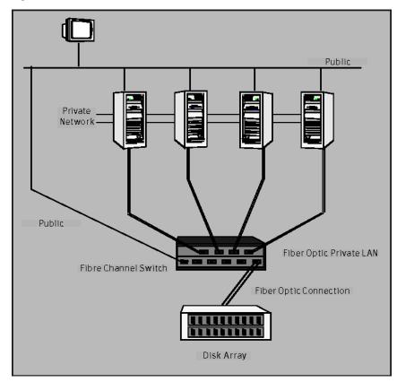
Four Node SFCFSHA Cluster Built on Fibre Channel Fabric Figure 3-1
