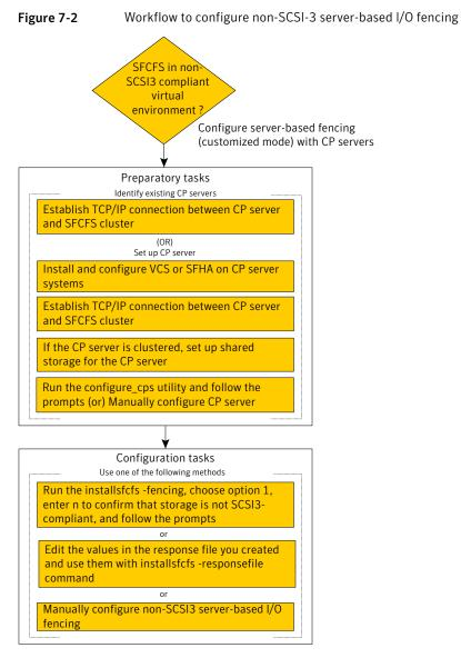
After you perform the preparatory tasks, you can use any of the following methods to configure I/O fencing:
