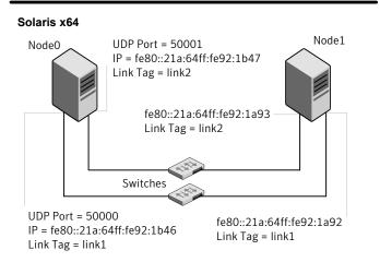
The configuration that the /etc/llttab file for Node 0 represents has directly attached crossover links. It might also have the links that are connected through a hub or switch. These links do not cross routers.
