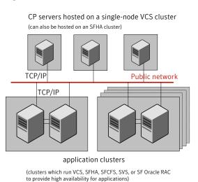
Figure 7-5 displays a configuration using a single CP server that is connected to multiple application clusters with each application cluster also using two coordinator disks.
