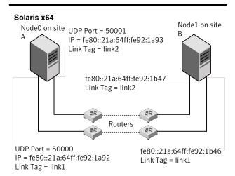
The configuration that the following /etc/llttab file represents for Node 1 has links crossing IP routers. Notice that IPv6 addresses are shown for each link on each peer node. In this configuration multicasts are disabled.
