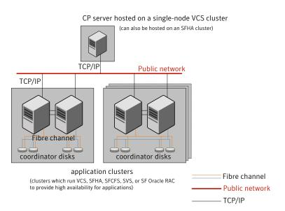
Figure 9-10 displays a configuration using a single CP server that is connected to multiple application clusters.
