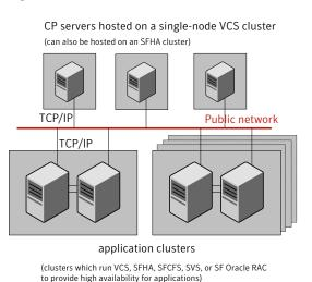
Figure 9-9 displays a configuration using a single CP server that is connected to multiple application clusters with each application cluster also using two coordinator disks.
