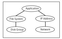
A single node can host any number of service groups, each providing a discrete service to networked clients. If the server crashes, all service groups on that node must be failed over elsewhere.
