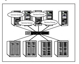
Figure 2-8 Shared disk architecture for basic cluster
