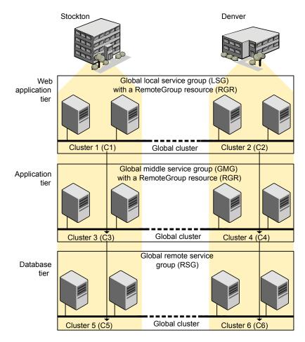
Figure 16-6 A three-tiered globally clustered application, database, and storage
