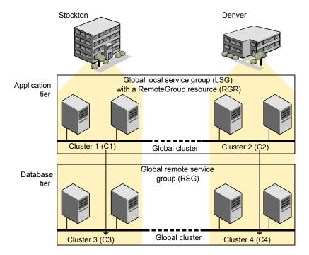
Just as a two-tier, two-site environment is possible, you can also tie a three-tier environment together.
