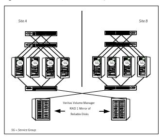
A campus cluster requires two independent network links for heartbeat, two storage arrays each providing highly available disks, and public network connectivity between buildings on same IP subnet. If the campus cluster setup resides on different subnets with one for each site, then use the VCS DNS agent to handle the network changes or issue the DNS changes manually.
