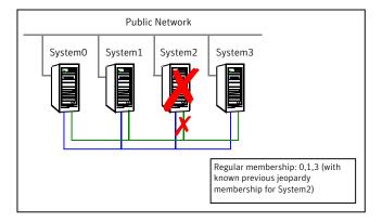
Systems 0, 1, and 3 recognize that System2 has faulted. The cluster is reformed. Systems 0, 1, and 3 are in a regular membership. When System2 went into jeopardy membership, service groups running on System2 were autodisabled. Even though the system is now completely failed, no other system can assume ownership of these service groups unless the system administrator manually clears the AutoDisabled flag on the service groups that were running on System2.
