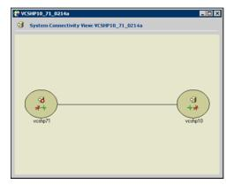
VCS monitors systems and their services over a private network. The systems communicate via heartbeats over an additional private network, which enables them to recognize which systems are active members of the cluster, which are joining or leaving the cluster, and which have failed.
