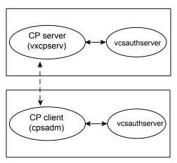
End-To-end communication flow with security enabled on CP server Figure 9-13 and VCS clusters
