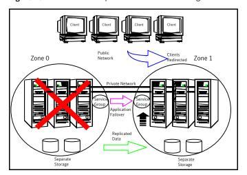
Figure 19-1 A VCS replicated data cluster configuration
