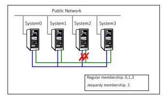
When a cluster interconnect link is re-established, all cluster status communications revert back to the cluster interconnect and the low priority link returns to sending heartbeat signal only. At this point, System2 is placed back in regular cluster membership.
