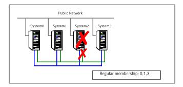
Systems 0, 1, and 3 recognize that System2 has faulted. The cluster is reformed. Systems 0, 1, and 3 are in a regular membership. The service groups on System2 that are configured for failover on system fault are attempted to be brought online on another target system, if one exists.
