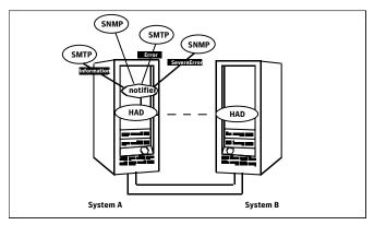
SNMP traps are forwarded to the SNMP console. Typically, traps are predefined for events such as service group or resource faults. You can use the hanotify utility to send additional traps.
