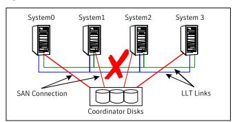
Figure 9-15 Four-system cluster where cluster interconnect fails
