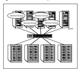
A dedicated, redundant server is no longer required in the configuration. Instead of N-to-1 configurations, you can use an N+1 configuration. In advanced N+1 configurations, an extra server in the cluster is spare capacity only.
