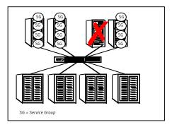
If any node fails, each instance is started on a different node. this action ensures that no single node becomes overloaded. This configuration is a logical evolution of N + 1; it provides cluster standby capacity instead of a standby server.
