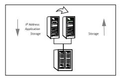
For example, in a two-node cluster consisting of db-server1 and db-server2, a virtual address may be called db-server. Clients access db-server and are unaware of which physical server hosts the db-server.
