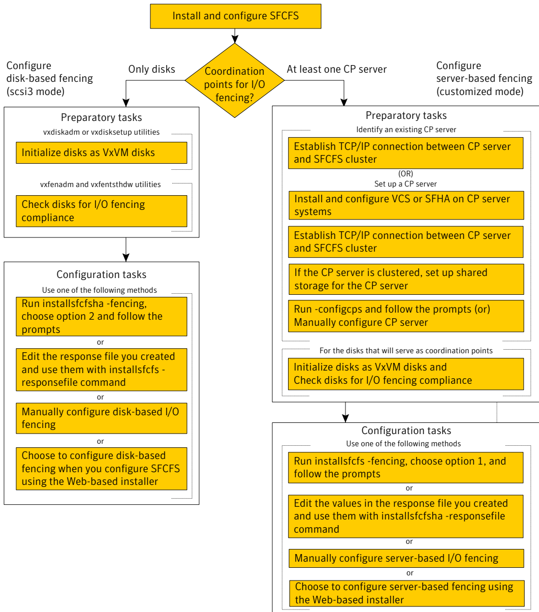
Figure 7-2 Illustrates a high-level flowchart to configure non-SCSI-3 server-based I/O fencing for the Storage Foundation Cluster File System High Availability cluster in virtual environments that do not support SCSI-3 PR.
