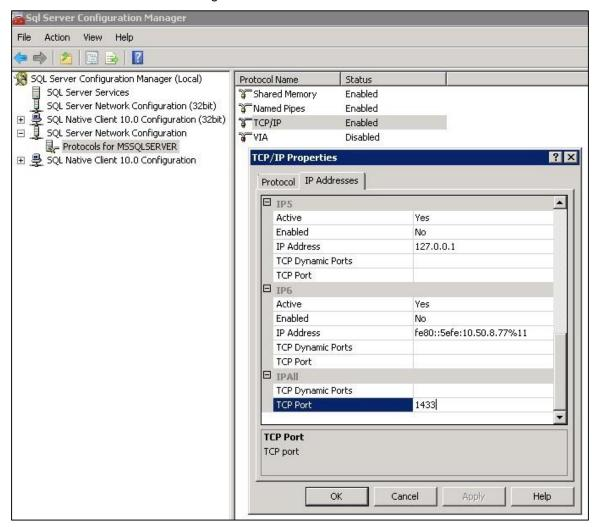
Figure 1: TCP/IP Properties
