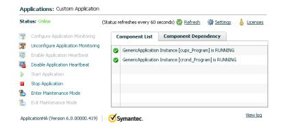
By default, the Component List tab appears. The tab lists each component of the configured application and the status description of each component.
