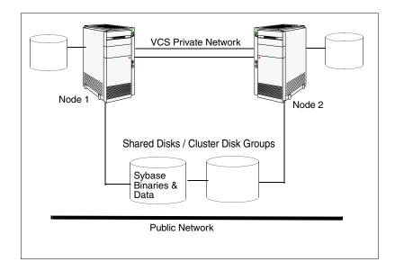
In the configuration depicted in the illustration below, the Sybase binaries are installed locally on each node in the cluster and the Sybase data is on shared disks or shared cluster disk groups managed using VxVM.
