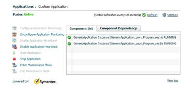
By default, the Component List tab appears. The tab lists each component of the configured application and the status description of each component.
