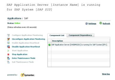
If the application status shows as not running, click **Start Application** to start the configured application on the machine.
