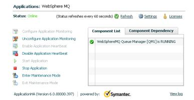
By default, the Component List tab appears. The tab lists each component of the configured application and the status description of each component.
