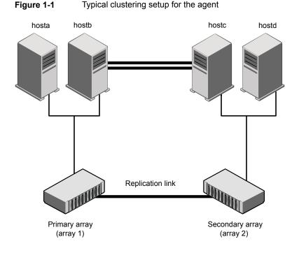
Figure 1-1 displays a typical cluster setup in a SRDF environment.
