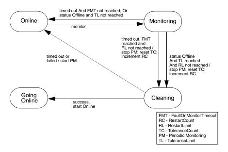
This diagram describes the activity that occurs when a resource faults and the RestartLimit is not reached. When the monitor entry point times out successively and FaultOnMonitorTimeout is reached, or monitor returns offline and the ToleranceLimit is reached, the agent invokes the clean entry point.
