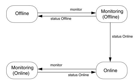
When resources are in a steady state of Online or Offline, they are monitored at regular intervals. The intervals are specified by the MonitorInterval parameter for a resource in the Online state and by the  ${\tt Offline Monitor Interval}\ parameter\ for\ a\ resource\ in\ the\ Offline\ state.\ An$ Online resource that is unexpectedly detected as Offline is considered to be faulted. Refer to diagrams describing faulted resources.
