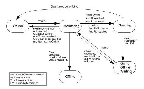
This diagram describes the activity that occurs when a resource faults and the RestartLimit is reached. When the monitor entry point times out successively and FaultOnMonitorTimeout is reached, or monitor returns offline and the ToleranceLimit is reached, the agent invokes the clean entry point.
