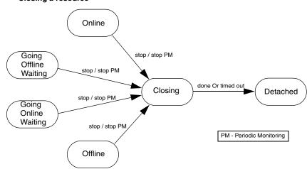
When the resource is disabled (Enabled=0), the agent stops Periodic Monitoring and the close entry point is invoked. When the close entry point succeeds or times out, the resource is placed in the Detached state.
