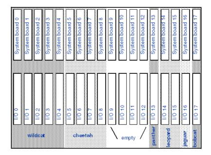
On Sun Fire 15K systems, system boards and I/O boards are numbered 0-17. On Sun Fire 12K systems, system boards and I/O boards are numbered 0-8. In the Sun Fire 15K example shown above, six domains have been configured, and there are additional empty slots.
