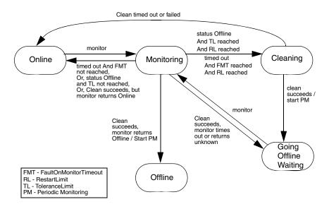
This diagram describes the activity that occurs when a resource faults and the RestartLimit is reached. When the *monitor* entry point times out successively and FaultOnMonitorTimeout is reached, or monitor returns offline and the ToleranceLimit is reached, the agent invokes the *clean* entry point.
