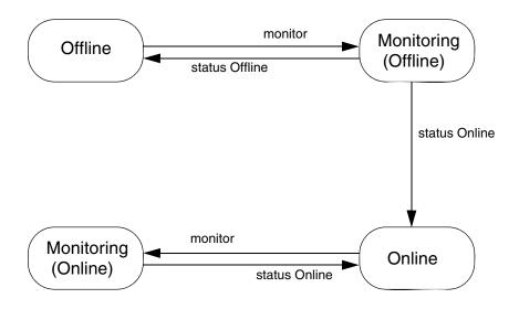
When resources are in a steady state of Online or Offline, they are monitored at regular intervals. The intervals are specified by the MonitorInterval parameter for a resource in the Online state and by the OfflineMonitorInterval parameter for a resource in the Offline state. An Online resource that is unexpectedly detected as Offline is considered to be faulted. Refer to diagrams describing faulted resources.
