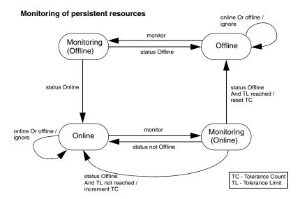
For a persistent resource in the Online state, if <code>monitor</code> returns a status of offline and the <code>ToleranceLimit</code> is not reached, the resource stays in an Online state. If <code>monitor</code> returns offline and the <code>ToleranceLimit</code> is reached, the resource is placed in an Offline state and noted as FAULTED. If <code>monitor</code> returns "not offline," the resource stays in an Online state.
