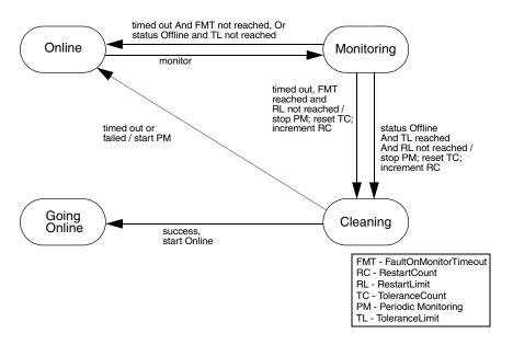
This diagram describes the activity that occurs when a resource faults and the RestartLimit is not reached. When the <code>monitor</code> entry point times out successively and FaultOnMonitorTimeout is reached, or monitor returns offline and the ToleranceLimit is reached, the agent invokes the <code>clean</code> entry point.
