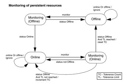
For a persistent resource in the Online state, if monitor returns a status of offline and the ToleranceLimit is not reached, the resource stays in an Online state. If monitor returns offline and the ToleranceLimit is reached, the resource is placed in an Offline state and noted as FAULTED. If monitor returns "not offline," the resource stays in an Online state.
