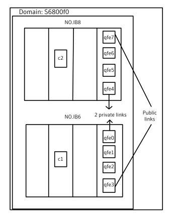
The highlights of the procedure to dynamically reconfigure the I/O boards (N0.IB8 board and IO15 board) in the wildcat and leopard domains for s6800 and e12K/15K/25K respectively include:
