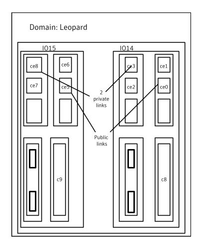
For e12K/15K/25K: In the following scenario, a cluster consists of the leopard and the S6800f0 domains. The cluster is running service groups on the leopard domain, which includes I/O boards IO14 and IO15. IO15 requires dynamic reconfiguration because of a malfunctioning component. The domain S6800f0 includes I/O boards IB8 and IB6. The disk controllers and NICs are labeled in the following diagrams.
