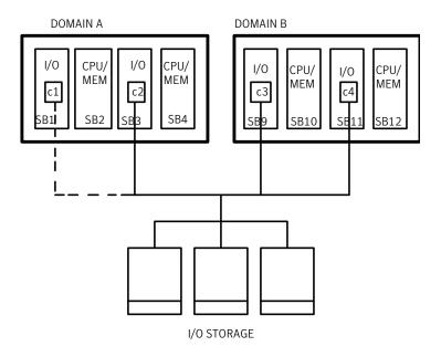
In the example, the system board SB3, which has a disk controller, is to be removed, repaired, and replaced. The administrator disables the controller, and the disk controller on SB1 automatically takes over because of the DMP functionality. Using dynamic reconfiguration commands, the administrator can detach, or remove the board from the Domain A's configuration. When this is complete, the board can be physically removed.
