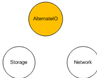
Figure 7-17 shows that the AlternatelO resource does not have any dependency on storage or network resources.
