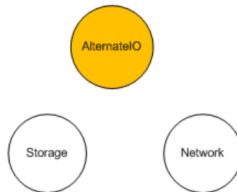
Figure 7-19 shows that the AlternatelO resource does not have any dependency on storage or network resources.
