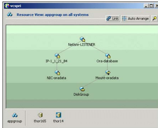
Figure 15-4 Example: A single-instance Oracle database is configured as a VCS service group (appgroup) on a two-node cluster
